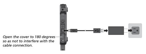
2. Power is being supplied from the external power source to MX50.
