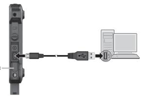
Open the cover to 180 degrees so as not to interfere with the cable connection.
