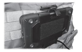
**NOTE:** The hinge of the mount might get loose after long time usage. Tighten the hex nut if this happens.
