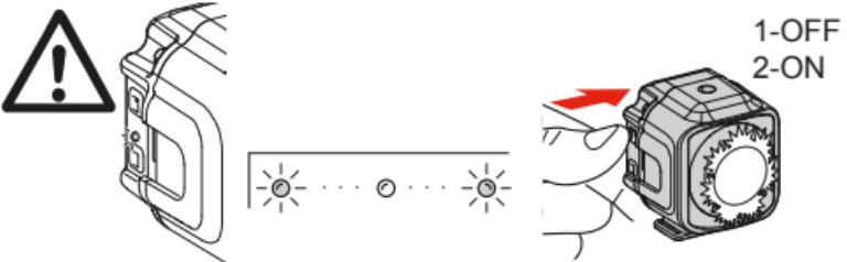
If the connection fails, the blue LED on the Beamo will start blinking. Please, restart your Smartphone App or turn the Beamo off and on again.
